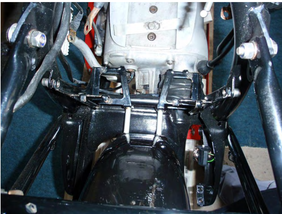
Bevel Drive with new rear wheel drive splines and vapour blasted
