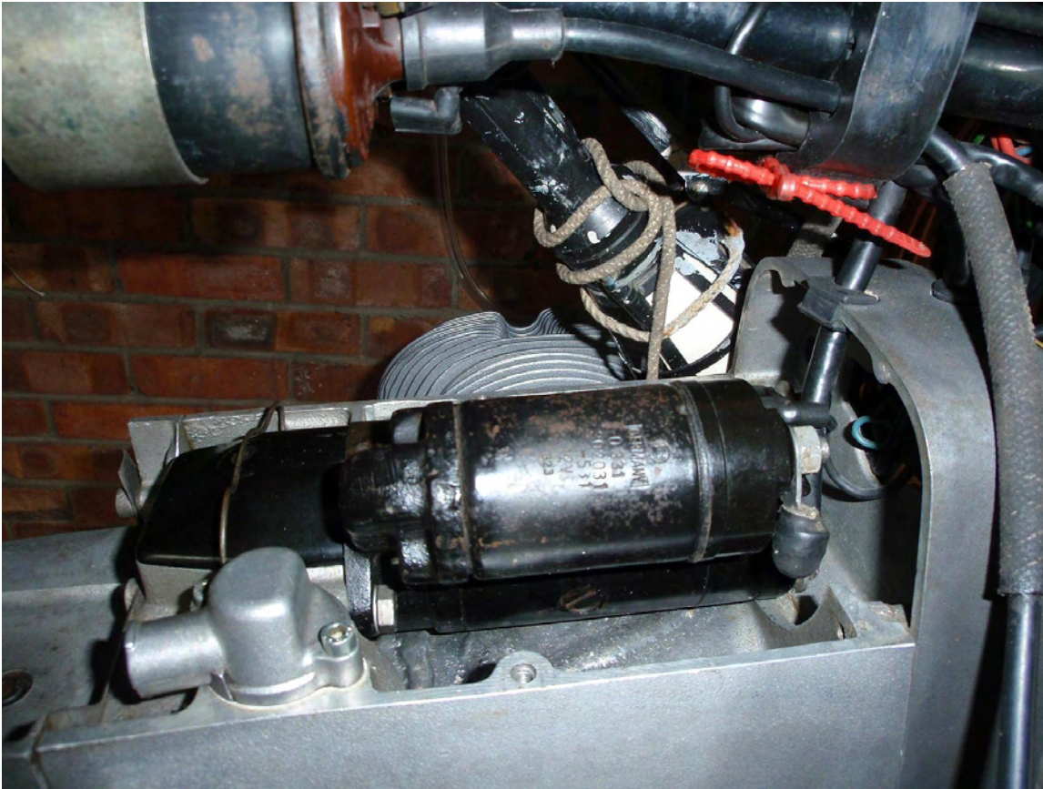
Air boxes (also vapour blasted) back on
