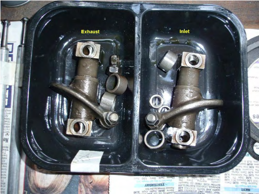
Here are the rockers off the LH head in their Tesco tray!
