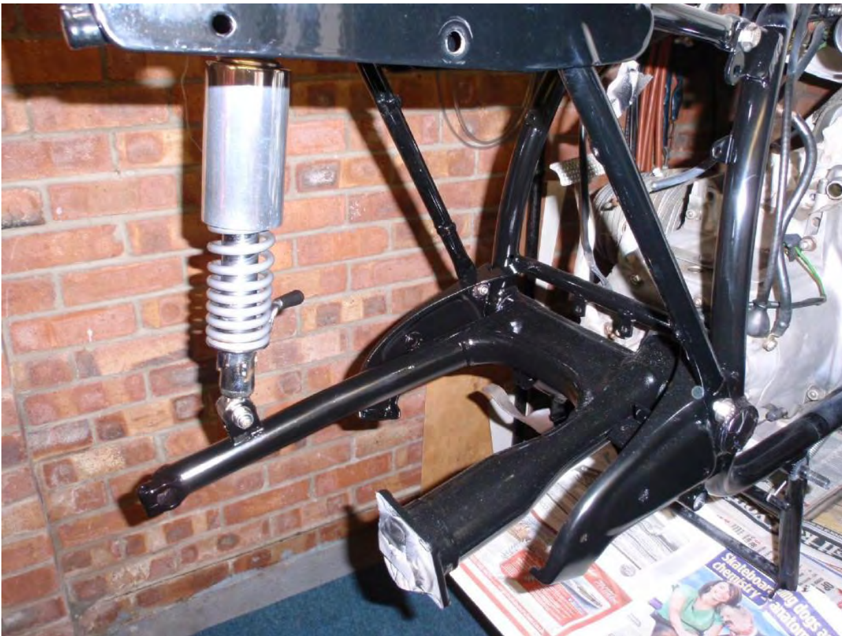
This shows the 2 coats of black gloss applied and removable frame refitted
