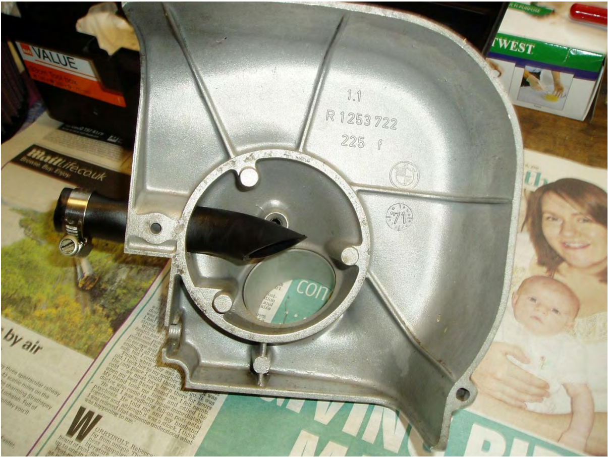
Photo below show correct route for breather pipe from crank reed valve.
